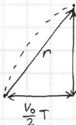
$$r = \sqrt{H^2 + \left(\frac{V_0 T}{2}\right)^2} = \sqrt{(g T^2 / 2)^2 + \left(\frac{g T^2}{2 \sin \alpha}\right)^2} = \frac{g T^2}{2} \sqrt{1 + \frac{1}{\sin^2 \alpha}} = \frac{g T^2}{2} \sqrt{\frac{\sin^2 \alpha + 1}{\sin^2 \alpha}} = \frac{g T^2}{2} \sqrt{\sin^2 \alpha + \sqrt{1 + \frac{4}{3}}} = \frac{g T^2}{2} \sqrt{\frac{4}{3}} = 20 \sqrt{\frac{4}{3}} \text{ м}$$
