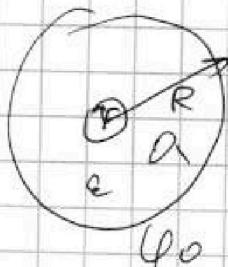
$$\varphi(t) = \frac{3}{2} \int_{B_0}^{\frac{B_0}{2}} S \sin \omega t \pi r^2 dr$$
