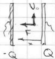
$$F = ma = \frac{Q}{C \cdot d} \cdot q \rightarrow a = \gamma \cdot \frac{Q}{C \cdot d} = \frac{v_0^2}{R}$$
