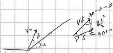
$$\frac{V_0 t}{\sin 90^\circ + \alpha} = \frac{S}{\sin 90^\circ - \alpha - \beta} = \frac{S}{\cos \alpha + \beta}$$
