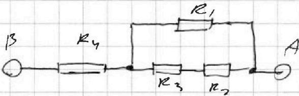
$$R_{23} = R_2 + R_3$$
