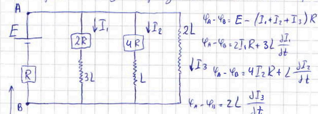
$$\varphi_A - \varphi_B = E - (I_1 + I_2 + I_3)R$$
