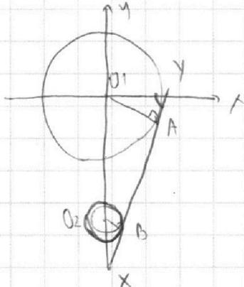
$$\triangle O_1AX \sim \triangle O_2BX \therefore K = \frac{O_1A}{O_2B} = \frac{5}{2}$$
