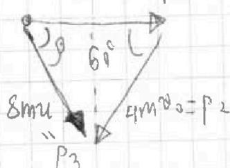
$$p_3^2 = 64m^2v_0^2 + 16m^2v_0^2 - 2 \cdot 8m^2v_0^2 \cdot 4 \cdot \cos 60^\circ$$
