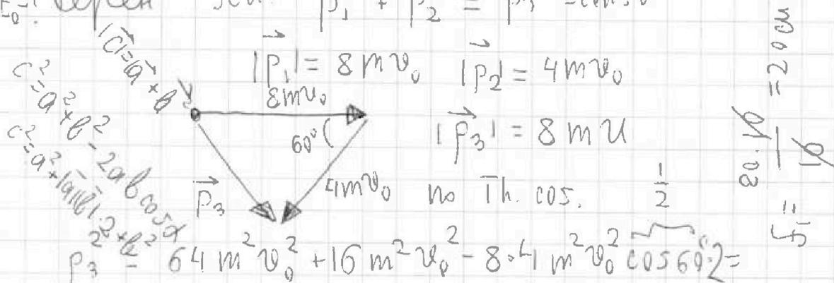
$p_3^2 = 64m^2v_0^2 + 16m^2v_0^2 - 8 \cdot 4m^2v_0^2 \cos 60^\circ =$
