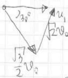
$$u_1^2 = 4v_0^2 + \frac{3}{4}v_0^2 - 2 \cdot 2v_0 \cdot \frac{\sqrt{3}}{2} v_0 \cdot \cos 30^\circ$$
