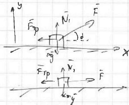
$$\left\{ \begin{array}{l} 1) \quad F \cos \alpha - \mu N_1 L = K \\ 2) \quad FL - \mu N_2 L = K \end{array} \right.$$
