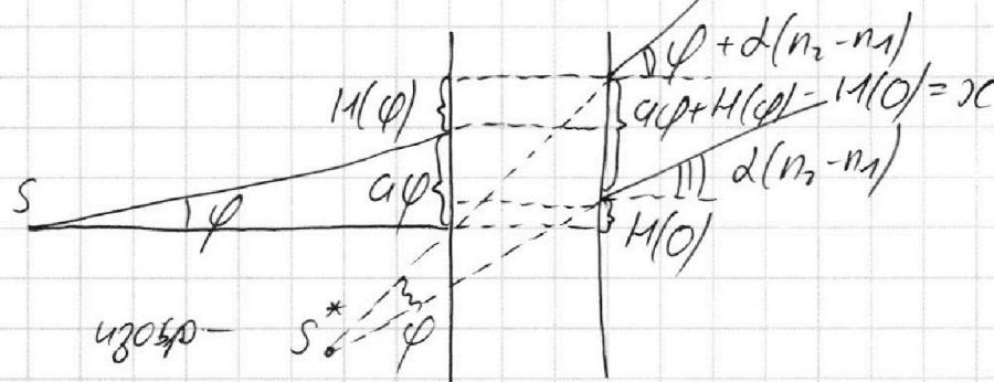
$$x = \alpha \varphi + H(\varphi) - H(0) = \alpha \varphi + h \cdot \frac{\varphi}{n_1}$$
