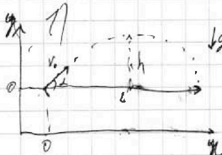
$$x = V_0 \cdot t \cdot \cos \alpha \quad x = L \quad L = \frac{V_0^2 \cdot \sin \alpha \cdot \cos \alpha}{g}$$
