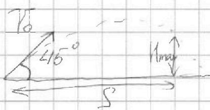
$$H_{\max} = \frac{S}{V_0^2} (V_0^2 - g S)$$
